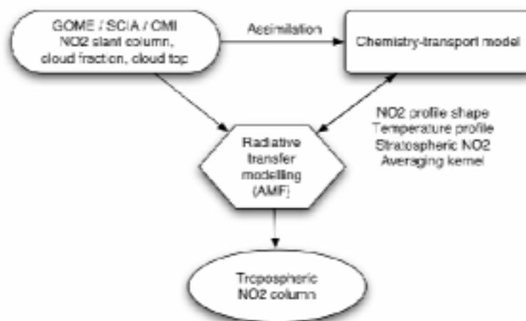
A major challenge is the derivation of high quality quantitative tropospheric NO<sub>2</sub> column amounts for individual ground pixels based on the satellite data. The retrieval of tropospheric trace gas species is characterised by large uncertainties, related to clouds, the surface albedo, the trace gas profile, the stratospheric column of NO<sub>2</sub>, and aerosols. Estimates of the retrieval uncertainties due to these aspects is non-trivial.
