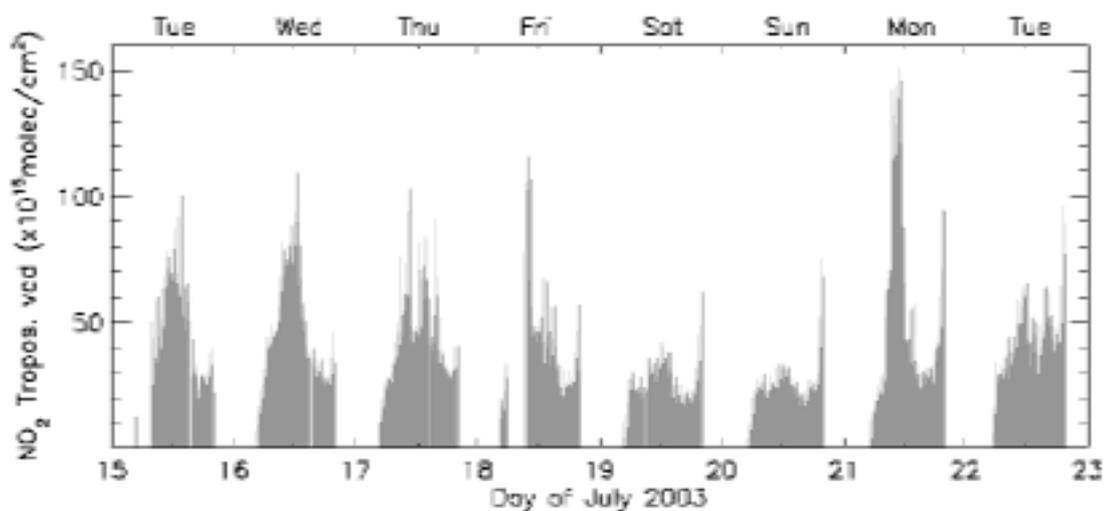
Figure 1: NO<sub>2</sub> column in the PBL (50-2165 m a.s.l.) observed in Bologna between 15th July 2003 and 22nd July, 2003.
