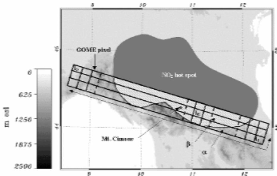
Figure 3. Illustration of the difference in representation of a satellite measurement, which is the NO<sub>2</sub> column over a large rectangle, and the ground measurement, which gives the NO<sub>2</sub> column over one specific location (picture provided by A. Petritoli, ISAC).
