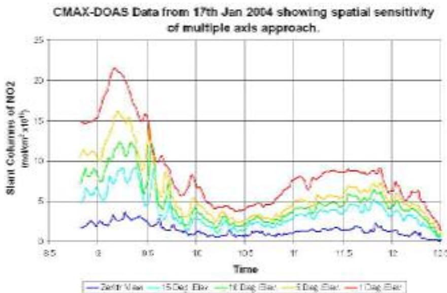
Figure 2: Slant Columns of nitrogen dioxide as measured by the Leicester CMAX-DOAS system, showing the detection of separate air masses (by resolving individual peaks), and providing an indication of dynamical motion (by the temporal shift in peaks)
