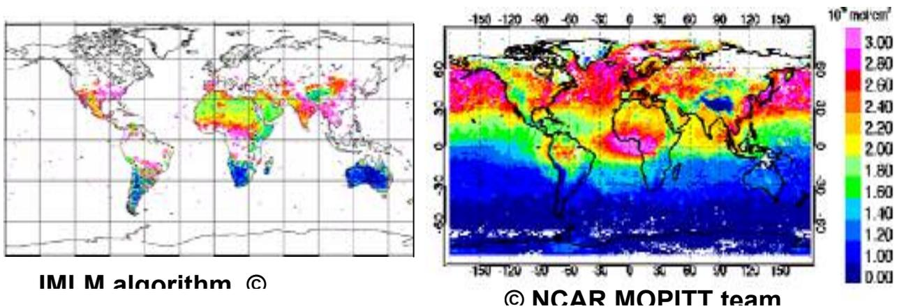
Figure 1: Global fields of monthly averaged SCIAMACHY CO retrieved with the IMLM algorithm for February 2004, compared with MOPITT CO for the same month.
