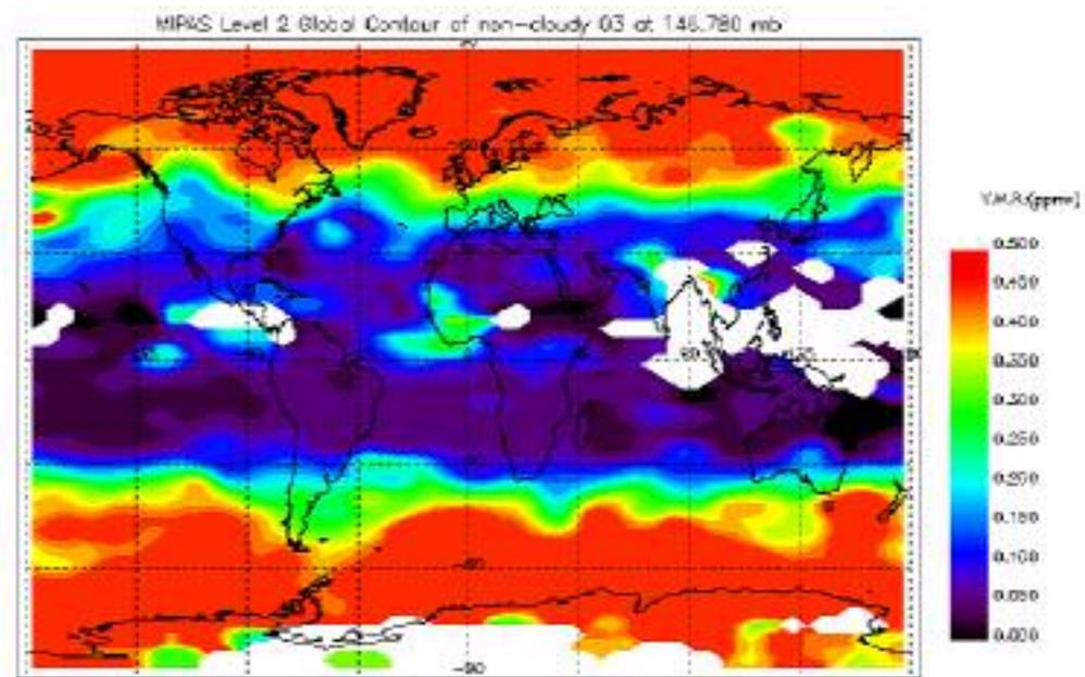
Figure 2. Global ozone at 146 mb (~13.5 km) measured by the MIPAS instrument for June to August 2003 (using operational near realtime level 2 data). White regions in the data are indicative of cloud-corrupted MIPAS data removed by the cloud detection system. Upper tropospheric concentrations over western Africa appear to reach as high as 0.35 ppmv indicating possible ozone enhancement due to biomass burning.
