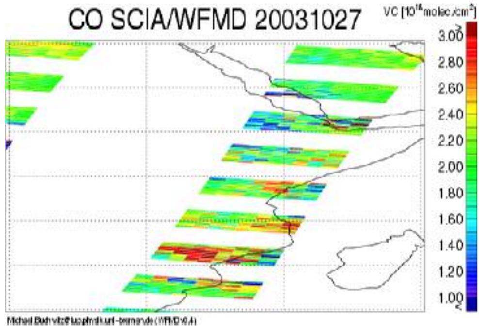
Figure 1. Enhanced concentrations of carbon monoxide (CO) due to biomass burning in eastern central Africa as retrieved by WFM-DOAS (Version 0.4) from SCIAMACHY near-infrared nadir spectra recorded on October 27, 2003 (Atmos. Chem. Phys., 4, 1954-1960, 2004).
