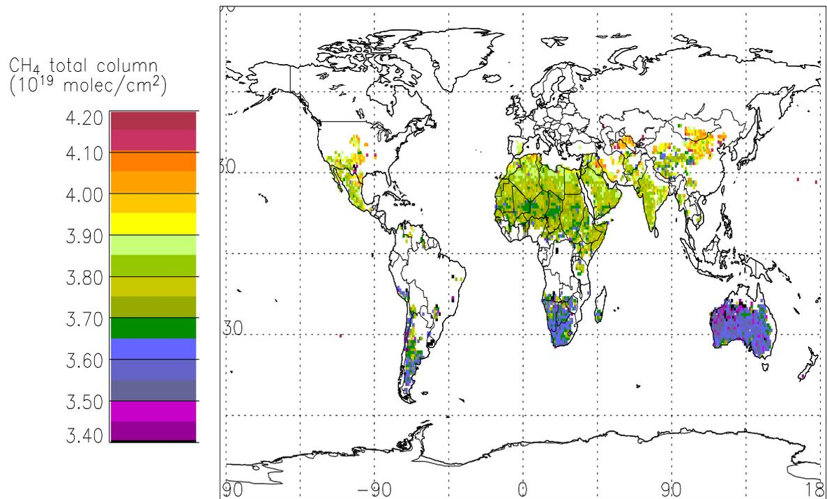
Figure 1. Monthly mean cloud-free CH<sub>4</sub> total columns for February 2004 from the SCIAMACHY IMLM algorithm normalised to the surface elevation (instrument related errors <math> < 0.8 \times 10^{18}</math> molec/cm<sup>2</sup>). [From: Straume *et al.* 2005, Advances in Space Research, Proceedings COSPAR 2004].
