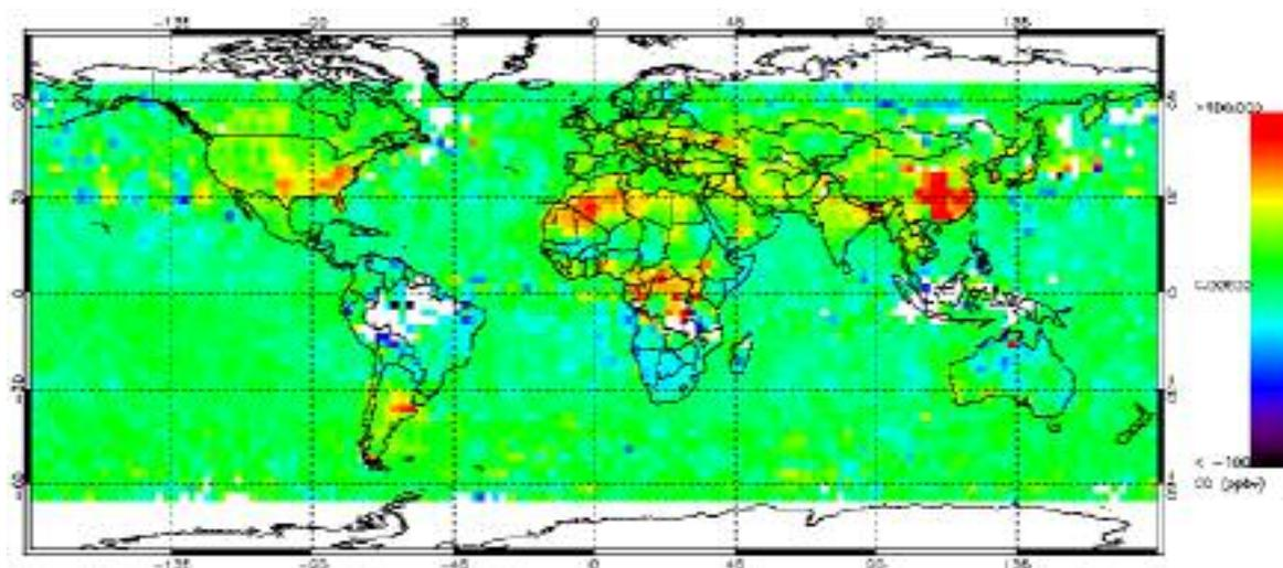
Figure 1. Monthly mean of MOPITT day-night “surface” concentrations for January 2001. Strong positive enhancements indicate high CO in the lowermost troposphere. Negative values may indicate high altitude (mid- to upper troposphere enhancements of CO).
